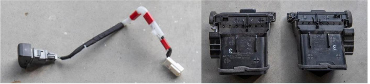
**F.Remove all the yellow/white plastic clips you can see from the back of the OEM Head unit and transfer them to the T10.**
