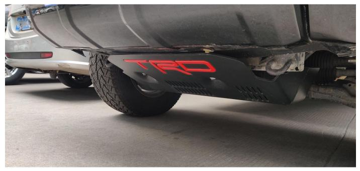
Note: If the front bolts are screwed in first, please do not tighten, then we screw the rear bolts into the holes, and finally tighten the 4 bolts separately.
