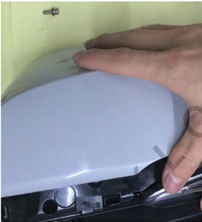
Install the rearview mirror bottom cover.
