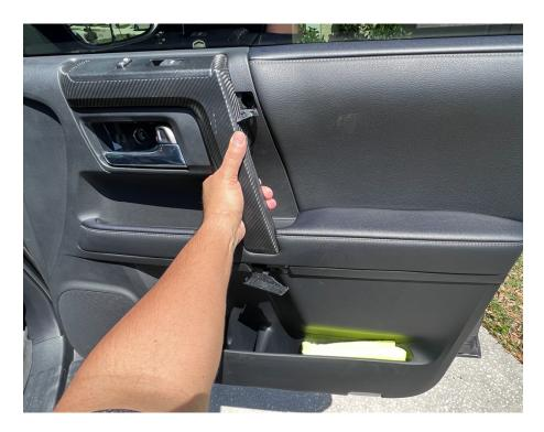
To remove the door panel, hold the door panel from the door handle and lift the panel a bit to separate the panel from the door frame. These are different kinds of snap-fit, so they'll pop off all simultaneously.
