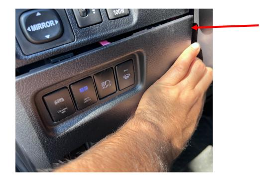
STEP 19. INSTALL NEW MIRROR CONTROL PANEL
