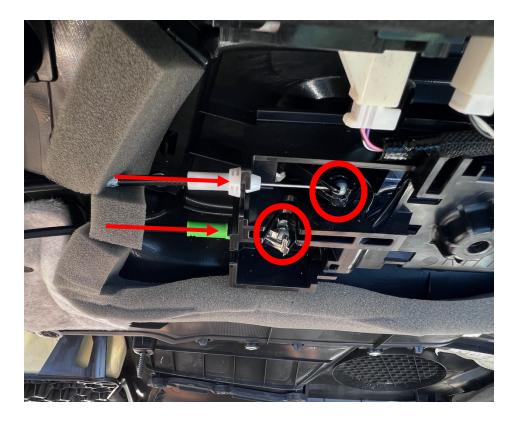
Also, there is a white and green Bowden cable termination. Carefully snap these out of the black housing and maneuver the steel cable ends out of their enclosures.
