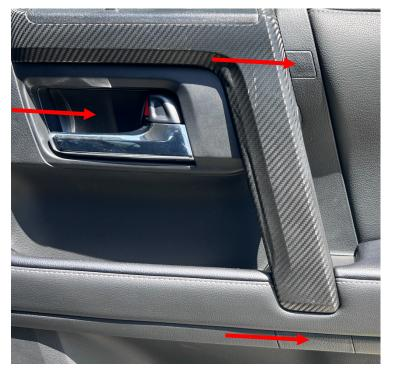
Using the trim removal tool, pry off the three marked s crew covers that hold the door panel in place.
