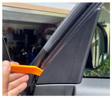
Starting on the driver-side door, pry off the mirror mount's plastic panel using an auto trim removal tool.
