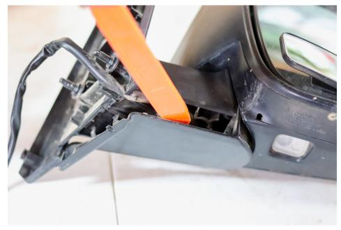
Using the trim removal tool, carefully pry open the lower mirror arm cover. It's a handful of snap fits, so be careful not to break any.
