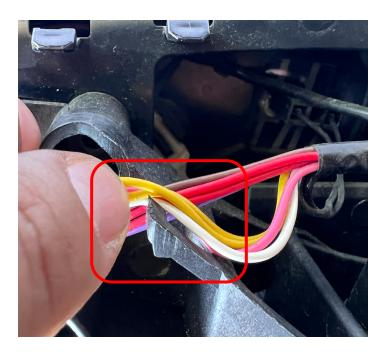
Remove the cables from the guide to get the arm loose.
