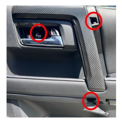
After opening the covers, remove the three screws using a Phillips screwdriver.
