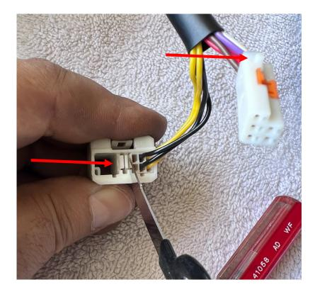
Looking closely at the entire connector, you'll notice four captive barbs on the outer sides and between the two internal connectors. These need to be pushed in to release the internal connectors from the external enclosure.
