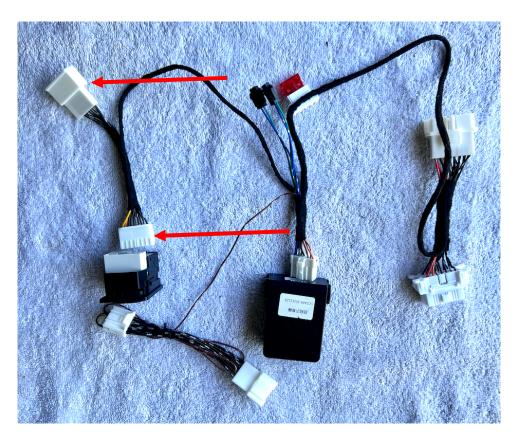
Plugin the intermediary harness; one side connects to the original connector, and the other side plugs into the new control module.
