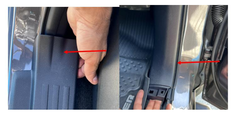
Removing some interior panels is necessary to access the wiring harness and the door grommet.
