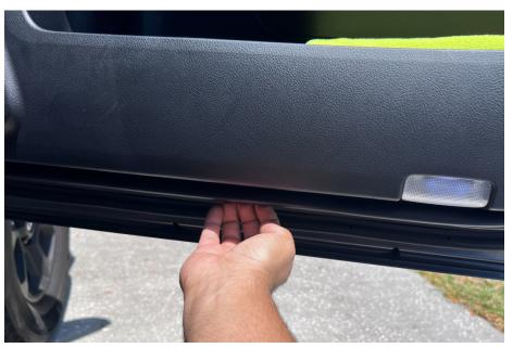
Using your hand or the trim removal tool, begin by pulling in the panel's lower side and separating the door panel from the door frame.
