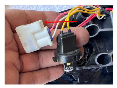
Looking at the assembly from the back, locate the white connector that needs to be unplugged by pressing the secure lock and twisting the puddle light base to remove the light bulb.
