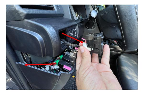
Pop open the dashboard by pulling on the top right corner of the lower panel, directly to the left of the steering column. You can reach up from below the current mirror control module and push it out from behind. Once it's out, disconnect the old control module by pressing the tab on the rear connector.
