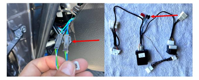
Use the included plug/receptacle pairs to connect the terminals from the power wires you just sent through the door grommets and the power wires from the mirror modules.
