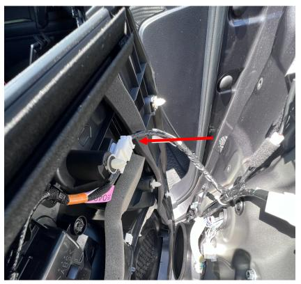
STEP 5. REMOVE DOOR CARD CONNECTIONS
