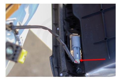
Before pulling the door panel apart, unplug the courtesy light connector located in the bottom left/right of the door panel. You'll have to slightly pull the bottom of the door panel away from the door frame to access the connector.
