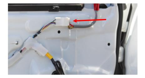
Now that we have the door frame exposed, we can easily find the mirror connector, follow the wire that's coming out of the mirror, and route down to the white connector at the top of the door.
