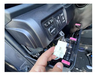
You can now install the new control module into the dashboard.
