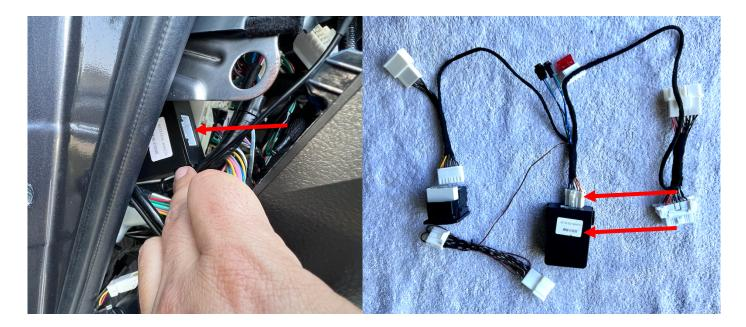
Peel the white paper from the Velcro and stick it to one side of the control box. Peel the other white paper from the other side of the Velcro and place the control box in the desired location (I put the control box by the open area close to the door.)
