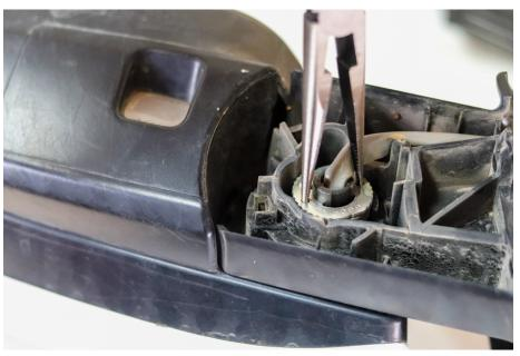
Use the needle-nose pliers for this step. The metal clip here keeps the mirror spring-loaded in open and closed detents. With the addition of the motor, this becomes unnecessary to get rid of it. Insert the tips of the needle-nose pliers into the two opposing holes on the spring clip.
