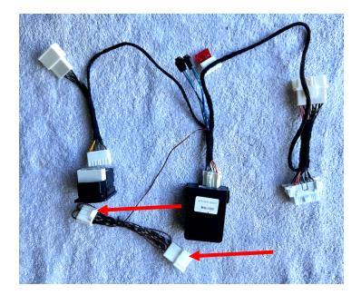
Find the connector pictured above (Kick panel) and remove the black connector by pressing the tab on the top. Plugin the intermediary harness; one side connects to the original female connector and the other plugs into the male connector.
