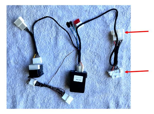
Remove the OBD connector from the frame by pressing the locks on both sides and connecting the intermediary harness. One side connects to the original connector, and the other side plugs into the new control module. Place the OBD side back into the frame.
