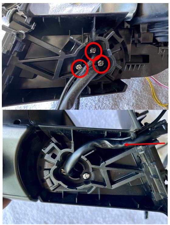
STEP 15. ASSEMBLE MIRROR ASSEMBLY TO MIRROR ARM
