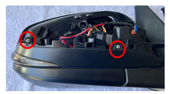
Remove the two screws and prim open the cover using the trim removal tool.
