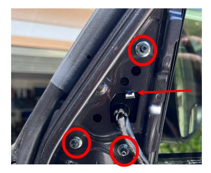
Unbolt the mirror assembly by removing the three 10mm nuts we exposed in **Step 1**. Carefully push down the plastic tab holding the mirror in place and pull the whole assembly out, cable and all.
