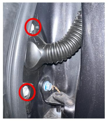
Open the door. This will expose two 10mm bolts that retain the wiring harness's bracket clamping. Undo these bolts and remove the tape securing the harness, giving you free access to the door grommet.
