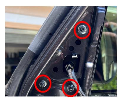
Once the cover is removed, you should see the three 10mm nuts that hold on to the mirror assembly.
