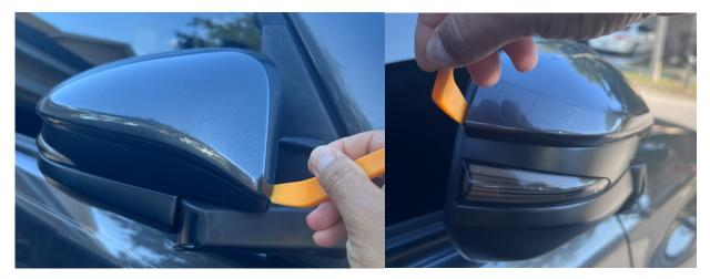
Another effective method to remove the cosmetic cover is folding the mirror and then pulling the bottom corner with one hand till the locks are loose.
