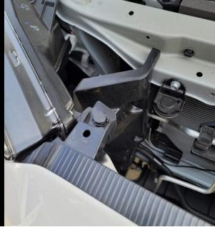
Next, pry the sides of the left and right bumper away from the inner fender skirt and this will expose the third headlight bolt:
