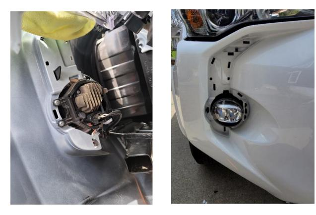
Now you can set the new DRL bezel in place. I ran the wires through this top hole making sure to keep the wires to one side when pushing the bumper back into place. There is a pressure clip that this spot attaches to, but is is much smaller than the actual opening so you don't need to worry about damaging the DRL wires:
