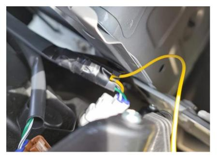
In the kit comes a controller box with 2 molex connectors, one is longer than the other. The longer side goes to the passenger DRL and the shorter to the driver DRL.
