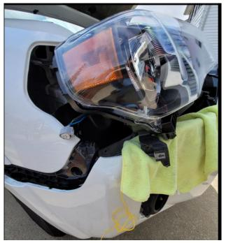
At this point with the bumper pulled forward you can also remove the old fog light trim ring. The clips have a tab that is easy to compress by hand then push forward through the front of the bumper. Start at the very top and work your way down.
