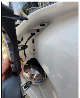
You can use a T-Tap wire connector to tap into the BLUE wire coming from the passenger side amber blinker bulb and the YELLOW wire coming from the driver side amber blinker bulb.
