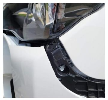
If working on the passenger side, remove the 3 bolts that hold in the headlight, as well as the push pin for that side mentioned in the last step, but leave the other push pin in the driver's side. This is what will hold your bumper from falling if you don't want to remove the whole thing.
