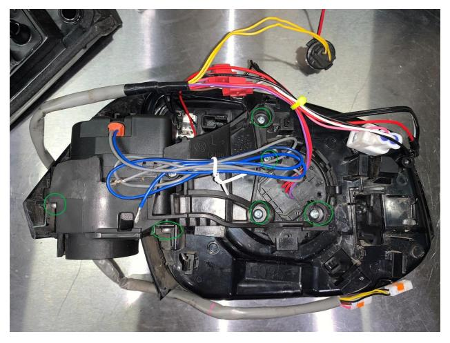
Install the motorized arm to the mirror housing. Reuse the original mirror screws.
