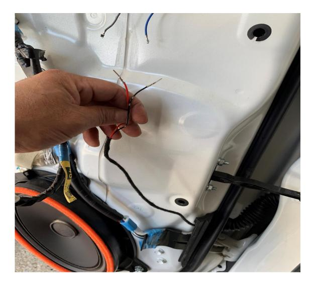
Now connect the pair of power wires to the mirror. Note the color of the wires. Harness side is red and black and mirror motor side is blue and grey.
