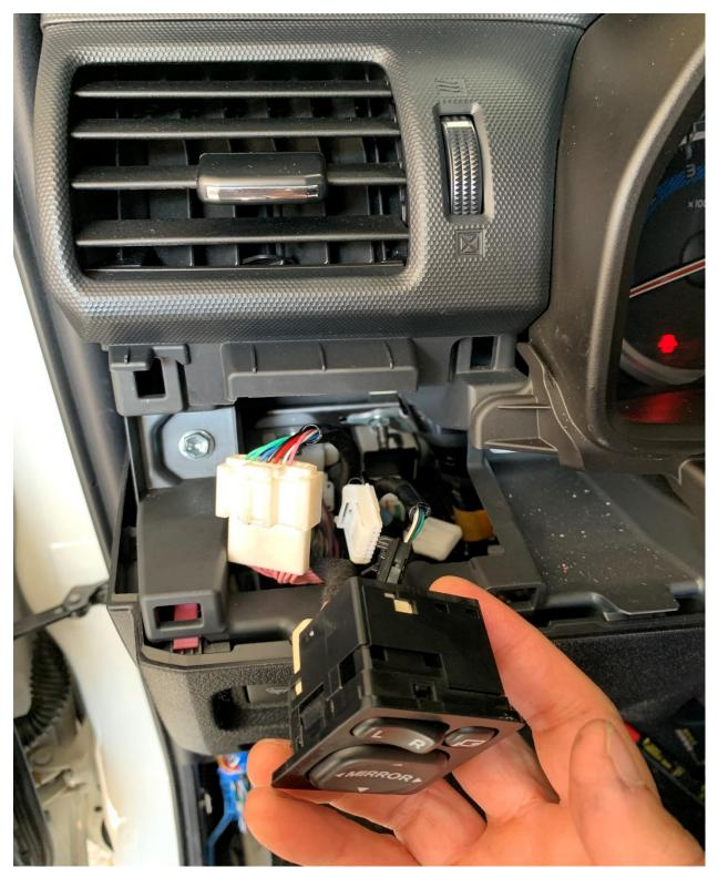
Installation is now complete. The mirrors should now fold when locked and unfold when unlocked. You can also manually fold/unfold the mirrors with the switch when the truck is on or in the accessory mode.
