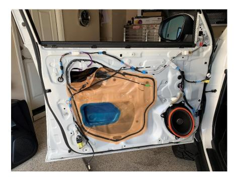
Remove these three nuts with a 10mm socket. Also remove clip on the rubber weather stripping.
