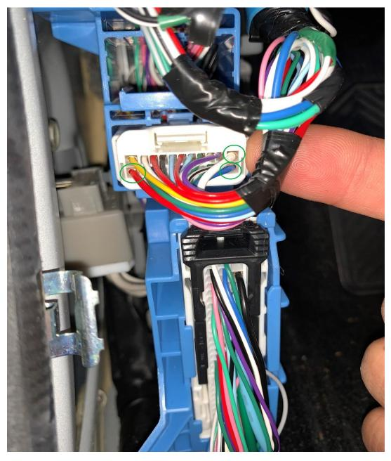
Connect harness wires to this connector. See the circled wires.
