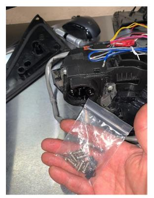
Line up up the 3 holes on the motorized arm with the mirror door base 3 holes. Screw in the 3 screws with the washers.
