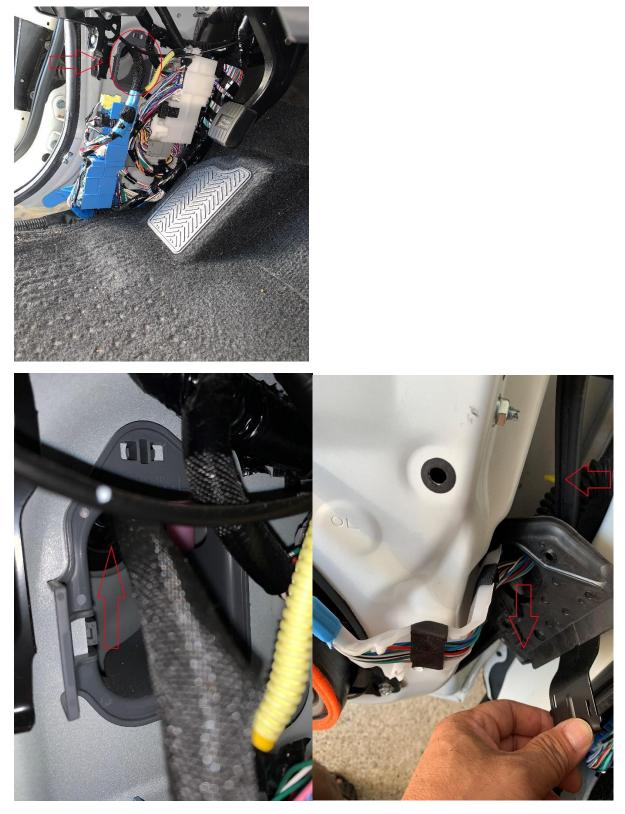
Route the power mirror part of the harness from the inside of the kick panel. Remove the rubber grommet, compress it and feed the wires. You may need to extend the power wires so it will reach the mirrors.
