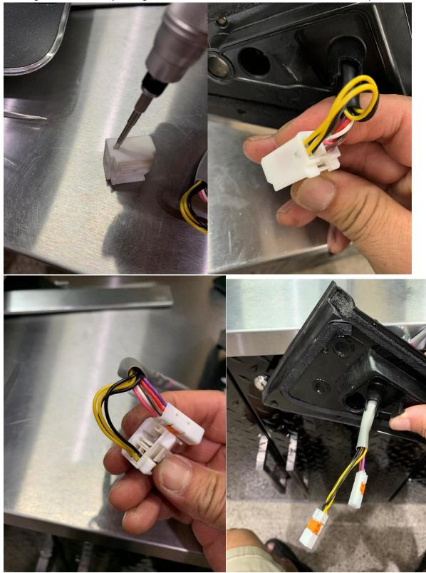
Pressing on this area and pressing the internal tabs to the sides will release the two clips.
