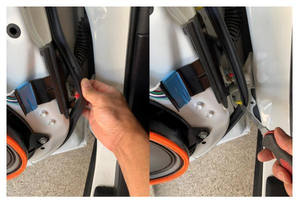
Remove these two 10mm bolts and remove the blue tape.
