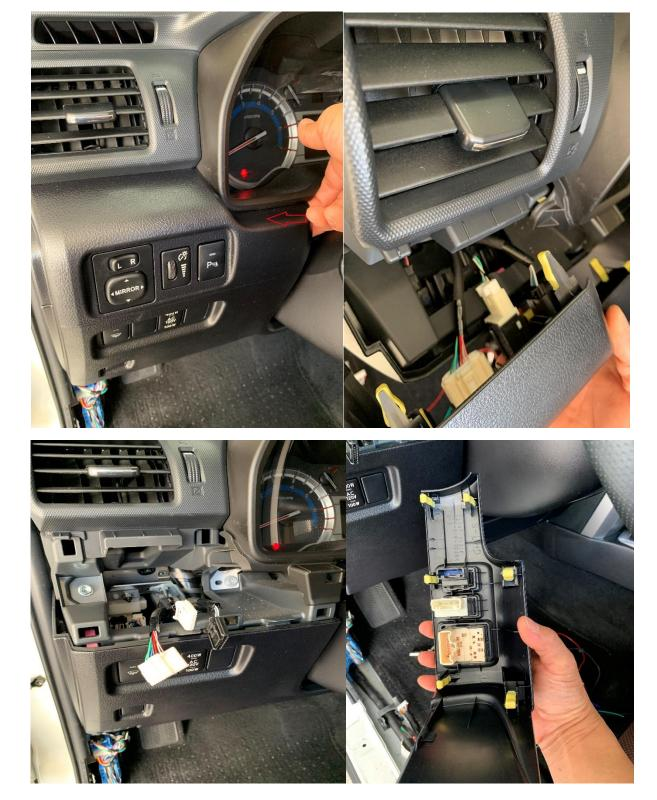
Remove the mirror switch cover. Pull this corner.
