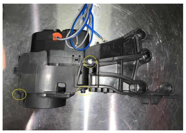
Before installing the motorzied mirror arm, remove these 3 screws. These screws will not be used.
