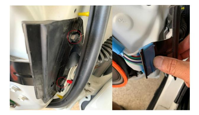
Remove the kick panel. Rotate the black knob counter clockwise and pull kick panel off. We need to route the part of folding mirror harness power wires (pick the shorter set of power wires) through the door grommet. Route only the pair of power wires
