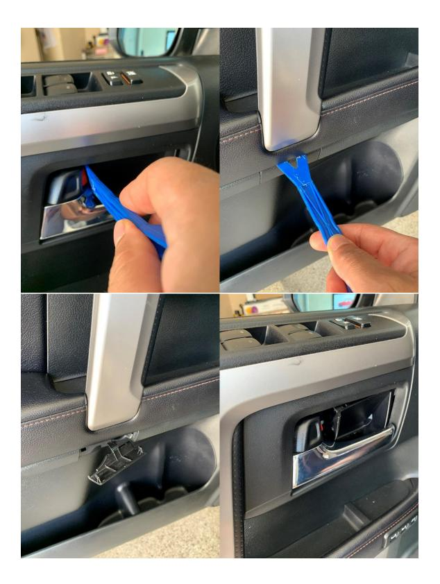
Once all 3 screws are out, pull on the edge of the door panel to remove.
