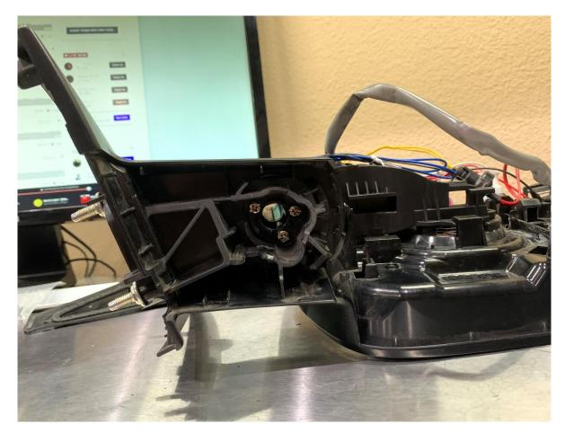
Feed the grey tubing and the two motor wires back into the motorized arm hole and also through the mirror base.
