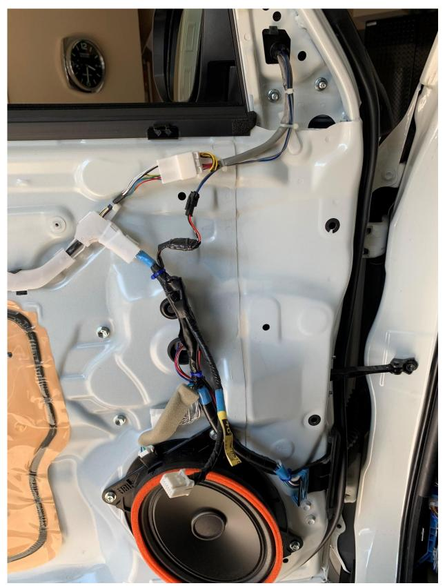
Use the provided connector to join the wires. Check orientation of the plugs before inserting.
